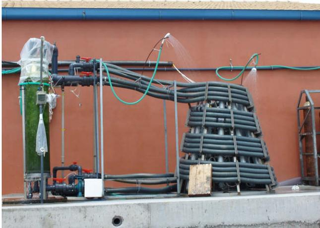
Fig. 3. Up-scaled experimental photobioreactor system in operation.
